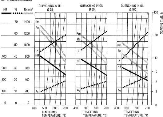
Hardening at 830—850°C with quenching in oil. Soaking time in minutes when the surface has attained full temperature, is 0.7 x thickness in mm. Interrupt the guenching at 125°C and temper immediately afterwards.
